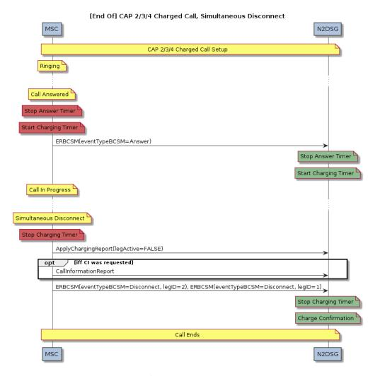
Figure W - CAP/INAP Flow (Simultaneous Disconnect)
