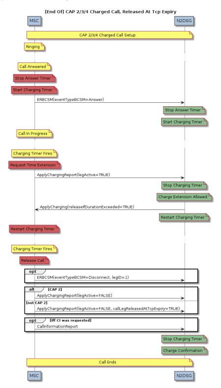
Figure Y - CAP/INAP Flow (Released at Tcp Expiry)
