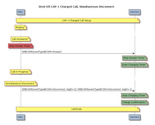
Figure QQ – CAP1 Flow (Simultaneous Disconnect)
