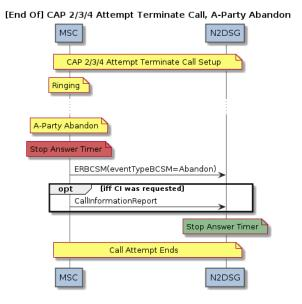
Figure F - CAP/INAP Flow (Attempt Terminate Abandon)
