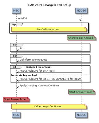
Figure L - CAP/INAP Flow (Charged Setup)
