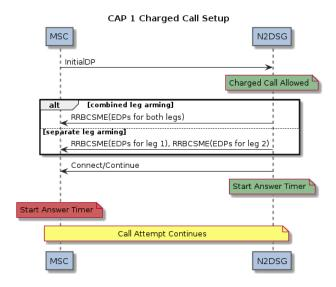
Figure MM – CAP1 Flow (Charged Setup)
