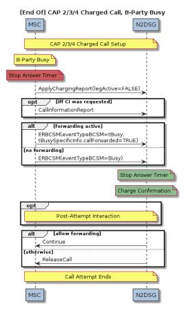
Figure N - CAP/INAP Flow (Charged Busy)
