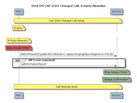
Figure P - CAP/INAP Flow (Charged Abandon)
