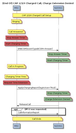
Figure R - CAP/INAP Flow (Extension Denied)
