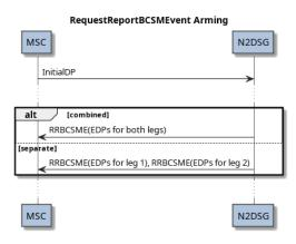
Figure DD - CAP/INAP Flow (RRBCSME Arming)
