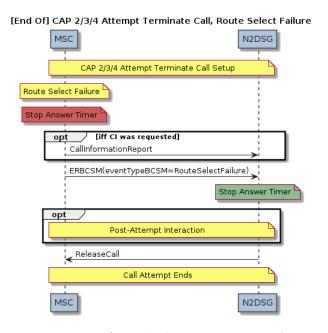
Figure C - CAP/INAP Flow (Attempt Terminate RSF)
