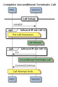
Figure A - CAP/INAP Flow (Unconditional Terminate)
