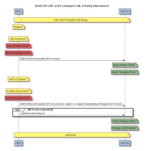
Figure S - CAP/INAP Flow (A-Party Disconnect)
