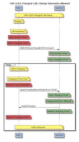
Figure Q - CAP/INAP Flow (Charged Call Extension Allowed)
