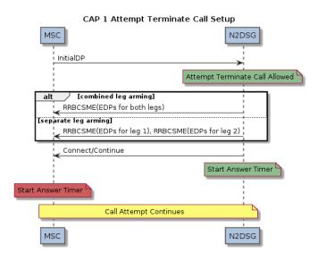
Figure GG – CAP1 Flow (Attempt Terminate Setup)
