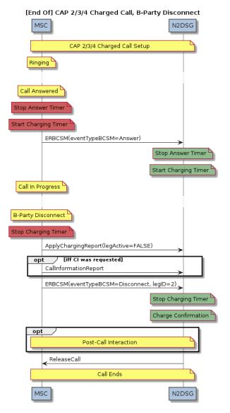
Figure U - CAP/INAP Flow (B-Party Disconnect)
