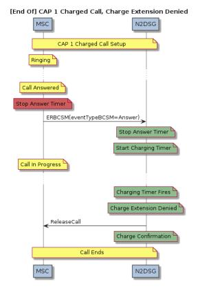
Figure NN – CAP1 Flow (Charged Call Extension Declined)
