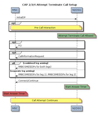
Figure B - CAP/INAP Flow (Attempt Terminate Setup)
