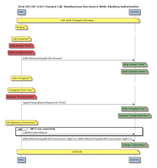
Figure X - CAP/INAP Flow (Simultaneous Disconnect Awaiting Authorization)
