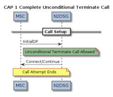
Figure FF - CAP1 Flow (Unconditional Terminate)
